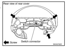
3. Remove screws (2) and remove switch and meter housing.
