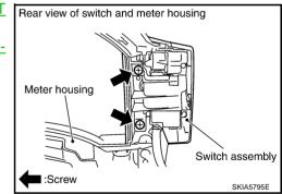
4. Remove screws (5), and remove odo/trip meter and illumination control switch.
