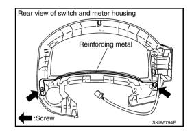
4. Remove screws (2) and remove reinforcing metal.
