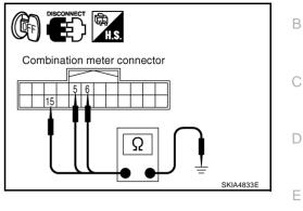
3. Check continuity between unified meter and A/C amp. harness connector terminals and ground.
